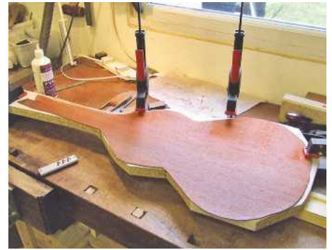
▲ Pic.9 The back needs to be scraped, then the braces can be glued on. Again, long-reach clamps will be needed for the brace middles
